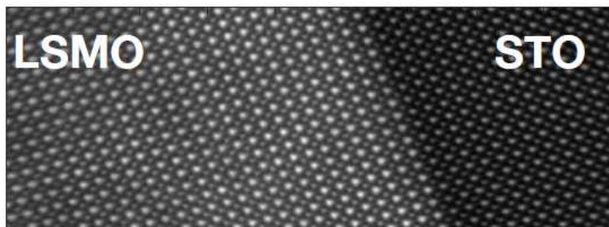
Figure 20: Cross-sectional transmission electron microscope image of our LSMO/STO thin films. While I do not claim it to be perfect, it is more uniform than the films in Figure 19.
